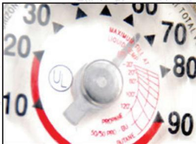
The gauge is located under the dome. The gauge will have numbers usually 5 to 95. The number on the gauge indicates the percentage of gas in the tank. (Some tanks have an additional pressure gauge. Don't be confused. Those numbers are from 0-300.)
